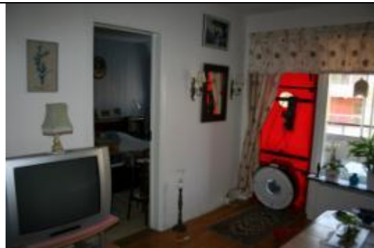
Figure 3a. The Blower Door was placed at the balcony opening.
