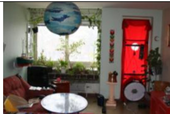
Figure 2b. Living room. Blower Door placed in opening for balcony door.
