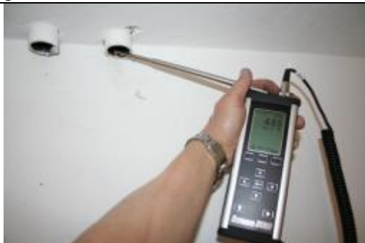
Figure 8a. Air speeds about 5 m/s was measured in pipe opening at an under pressure of 50 Pa. Air temperatures was measured to +14°C, which indicates that it is outdoor air and not air from neighbor apartment.
