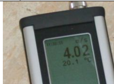
Figure 11a. Supply air device in bed room was temporary sealed with glass wool and foam plastic. Without sealing was an air speed of 4 m/s measured in the opening and an air temperature of +20°C, which indicates that it is air from neighbor apartment.
