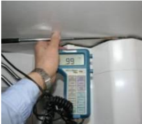
Figure 3. Leakage flows from neighbouring apartments and other areas were located by feeling with a hand and with smoke bottles (RFA) and air velocity meters (TSI).
